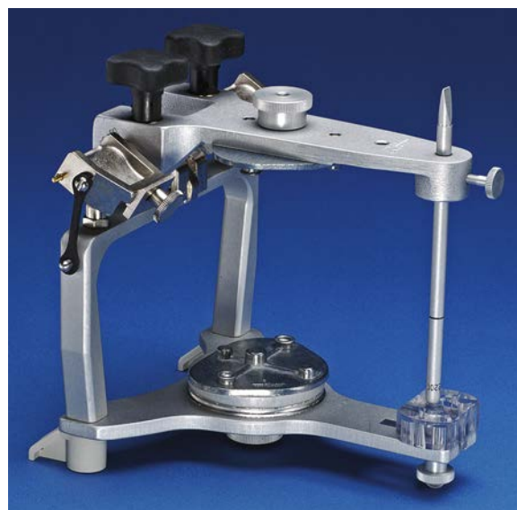
• Fig. 18.8. A semiadjustable articulator (Whip-Mix 2000 series Model 2240, Whip-Mix Inc., Louisville, KY.)
